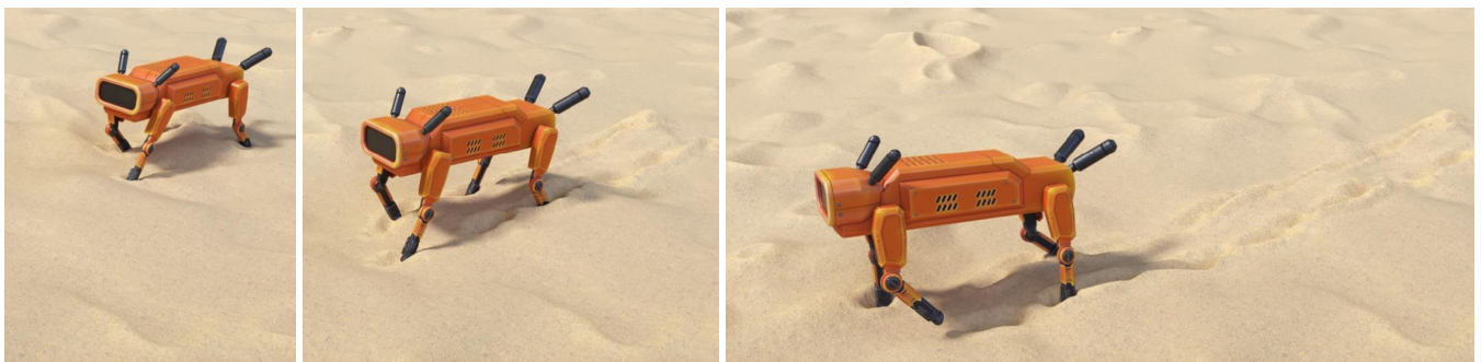
Figure 1: Robotic dog. Our method offers a real-time simulation solution for multibody systems with intricate joints and contact. The simulation of a quadrupedal robotic dog walking on sandy terrain achieves a frame rate of 56 FPS.
