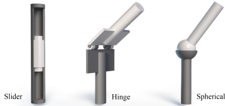
Figure 2: Illustration of three lower pairs: slider, hinge and spherical joints.
