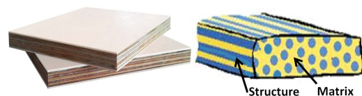
Figure 1: Composite materials are made of two or more constituent materials with different mechanical behaviors and are used in engineering(left). The simplified model we use is made of a based matrix and embedded fibers.(right)
